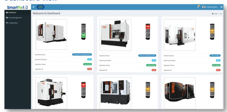
Representation of a machines on floor along with status indicators derived from sensor data.
